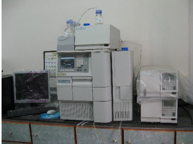
Figure 6 High Performance Liquid Chromatograph (HPLC) – for specific analyses
