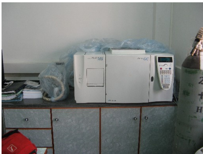
Figure 8 Mass Spectrometer and Gas Chromatograph for detection of contaminants of food and water
