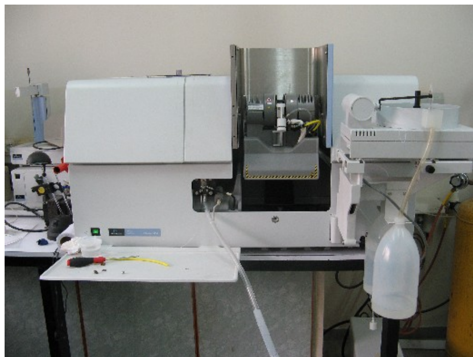
Figures 10a,b,c,d,e Mr Sami Lubbad working on a Perkin Elmer Atomic Absorption Instrument
