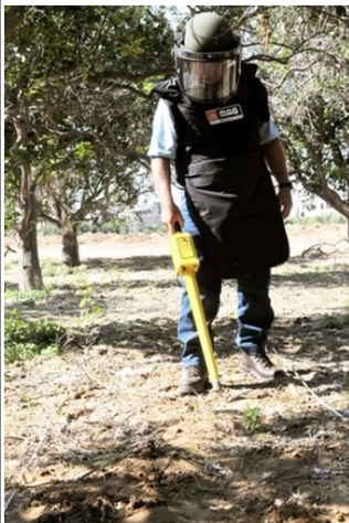
Specialist detectors donated by Schonstedt enable MAG EOD teams to search beneath the ground surface and ease the search between and around the rubble.
