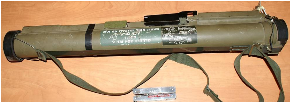
Typical shoulder-fired rocket in launcher, moving might actuate the trigger mechanism
