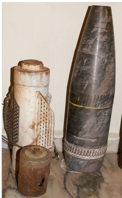
155 mm ILL, note illumination charge cont.
