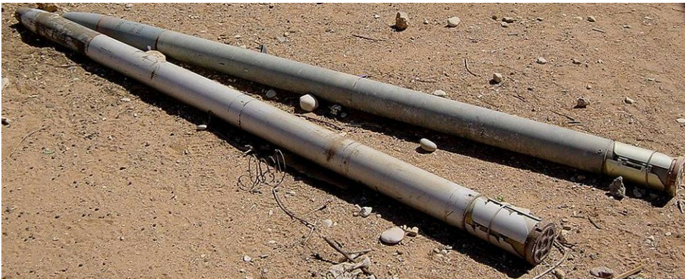
Typical ground-to-ground rocket system, contains HE-warhead and explosive propellant
