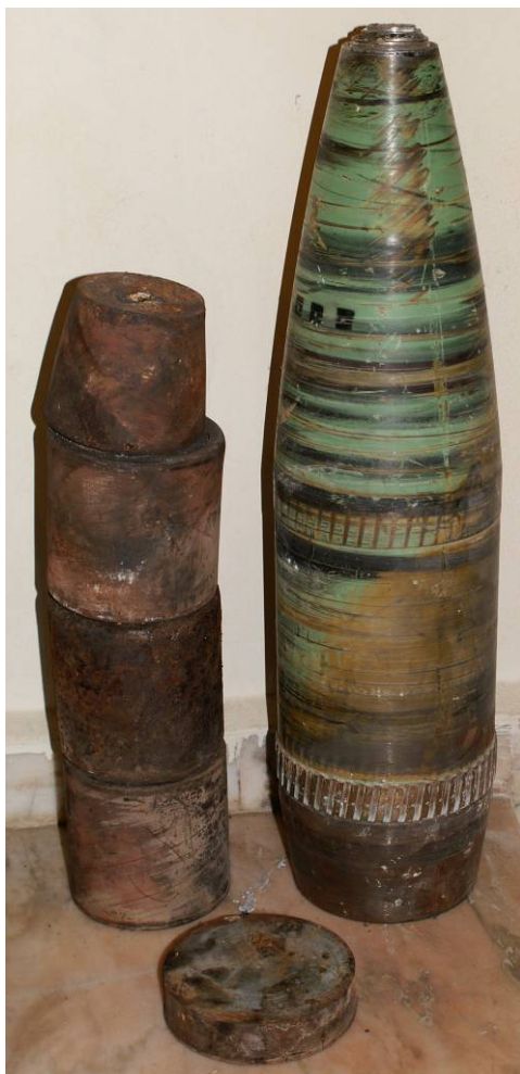
155 mm SMK HC, note smoke canisters
