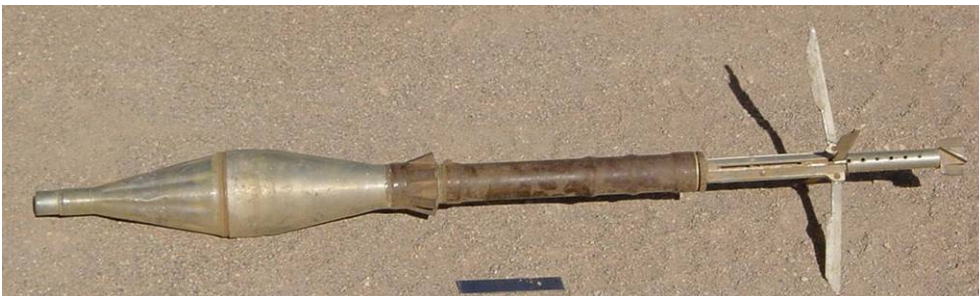
Typical shoulder-fired rocket, moving might actuate extremely sensitive fuze
