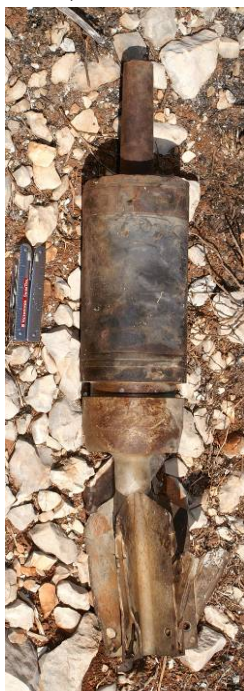
120 mm HEAT, fin stabilised
